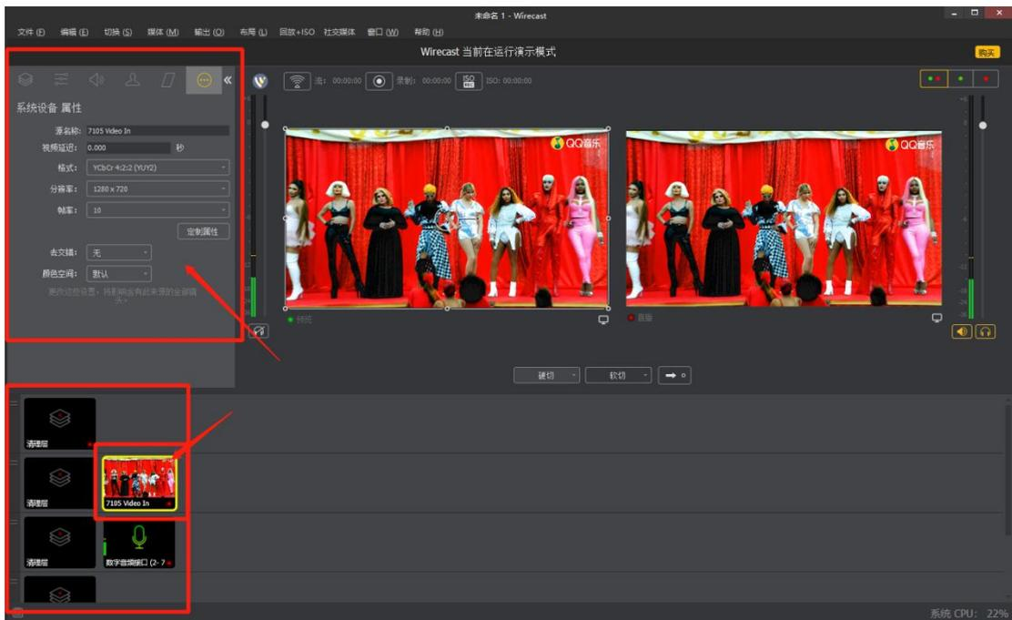
Note: Wirecast captures HDS7105 video, the video format only supports YUV, and the maximum resolution is 1280X720.
